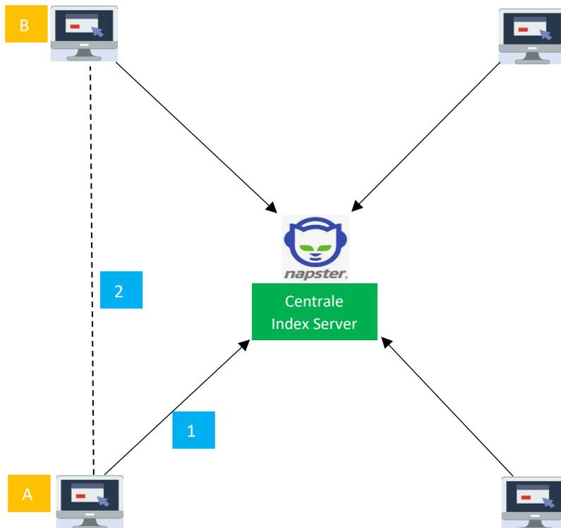
Figure 5: Napster network. (1) Computer A performs a search on Napster's central index server for Michael Jackson - Billy Jean. Napster's central index server looks for computers connected to the network that have the number available on their hard drive. (2) Computer B has the number. Laying computers A and B a direct peer-to-peer connection, after which computer A downloads the music file from computer B.
