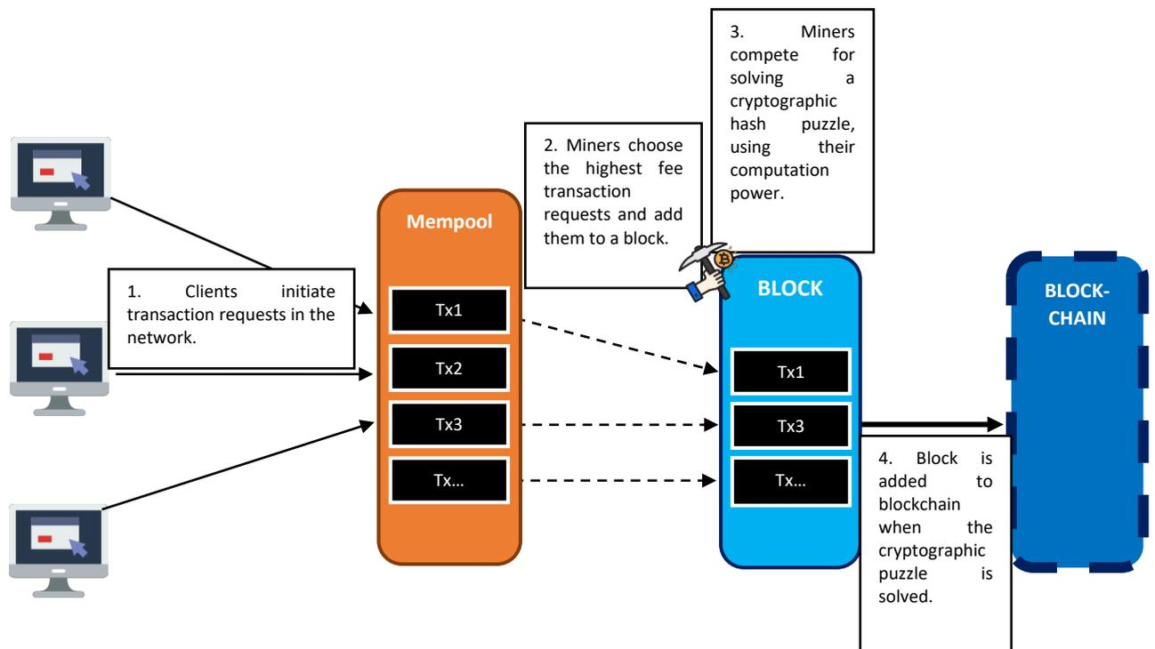
Figure 7: Schematic representation of how a transaction is added to the Blockchain. The mempool is where unconfirmed transactions come in and are kept. Miners choose which of the transactions from the mempool they want to add to the block. Subsequently, they try to solve a cryptographic puzzle. Once solved, they receive a block reward in bitcoins. (Source: Book: Lin Lim, C., Janse, A., *Blockchain Basics*, 2021, chapter 4).
