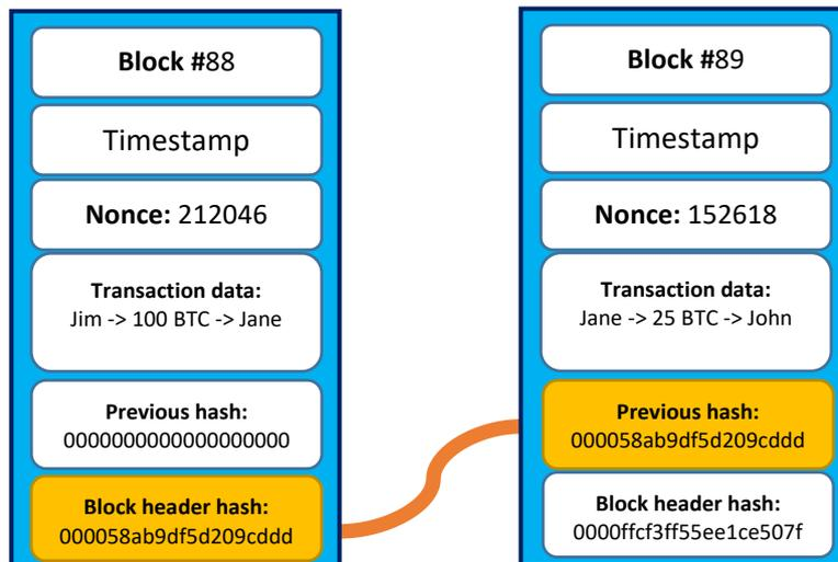
Figure 6: Simplified representation of a valid genesis block and block #2 with both blocks chained together using the block header hash and the previous hash. (Source: Lin Lim, C., Janse, A., *Blockchain Basics*, 2021, chapter 3).
